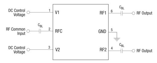
$C_{\rm BL}$  = 47 pF for >1 GHz operation. Increase value for lower frequency operation.
