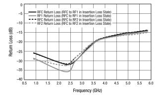
Figure 5. Return Loss vs Frequency (Insertion Loss State)
