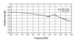
**Figure 3. Typical Insertion Loss vs Frequency**
