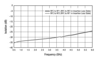
**Figure 4. Typical Isolation vs Frequency**
