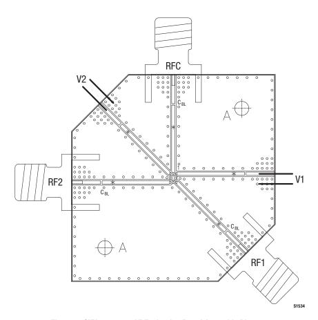
Figure 8. SKY13370-374LF Evaluation Board Assembly Diagram
