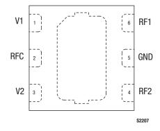
Figure 2. SKY13370-374LF Pinout – 6-Pin DFN (Top View)
