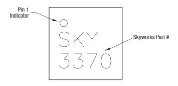
Figure 10. Typical Part Markings (Top View)
