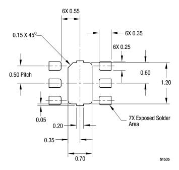
Figure 9. SKY13370-374LF PCB Layout Footprint (Top View)
